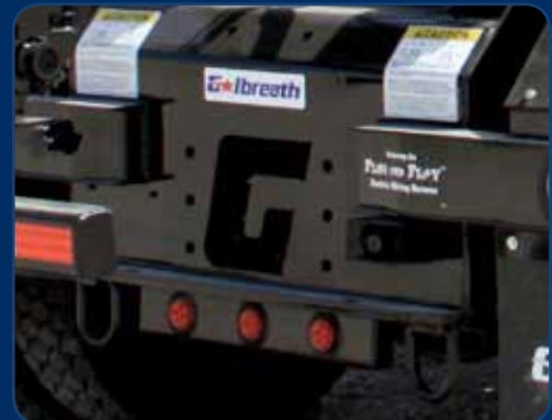
Pintle ready rear aprons allow for the addition of a pintle hook and easy upgrade to a trailer package
