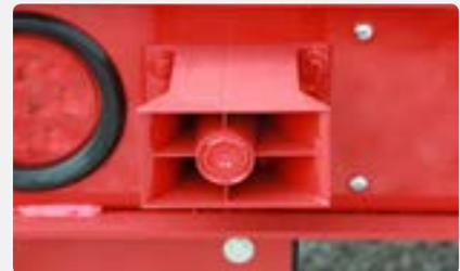
The hoist-up alarm is a standard safety feature. When hoist is engaged, alarm will sound, warning of hoist and container movement.
