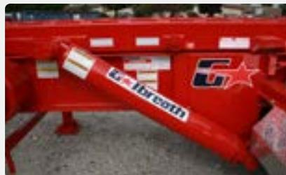
2 cylinders are mounted on the outside of the rails to provide stability when loading heavy boxes.
