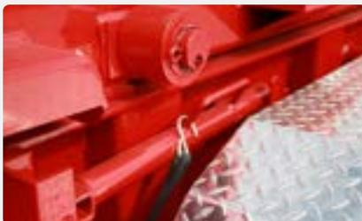
All trailer hoists have a safety prop to add extra security when the hoist is in the up position. 4 rollers per side help aid the container as it is loaded or unloaded on the hoist. Each roller is equipped with a bearing and a grease fitting for easy rolling and maintenance.
